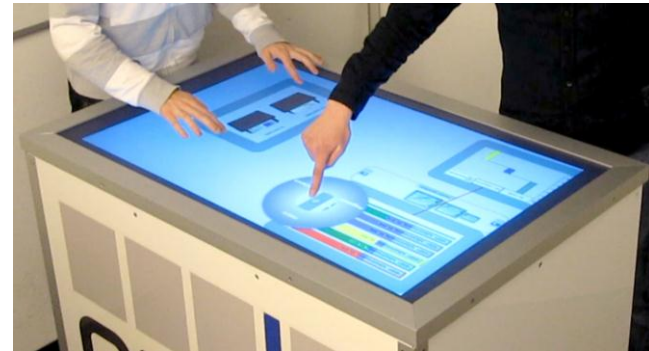
Figure 1. Two users simultaneously interacting with an interactive tabletop (120 x 80 cm). Note that users stand at different positions at the table. Users interact with objects, which are orientated towards them, are placed in a reachable position, and are scaled appropriately to enable proper interaction by touch.
