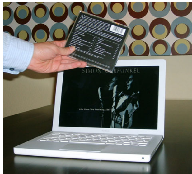
Fig. 4 A CD in front of the computer's webcam is recognized and the associated music is started
